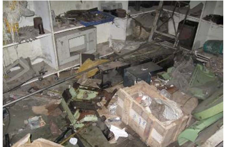
No protection to prevent damage and rust
