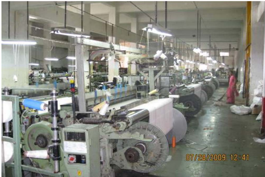
(3) Weaving the fabric on the weaving loom
