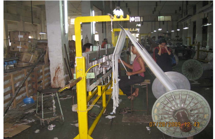
(2) Drawing the warp beam ready for weaving
